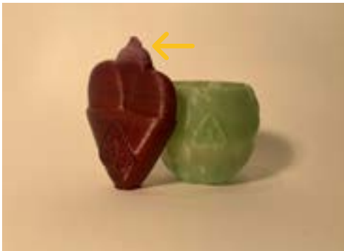
Picture18: Failed prints: left is caused by too much detail in the top, the material has no time to cool and cristalyzes, and left was caused by a clogged nozzle.
