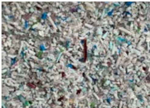
Picture 9: Granules from the shredded filament, giving it a rounder shape with more material volume.
