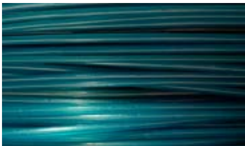
Picture 14: A good example of spooled filament. Consistent diameter and perfectly aligned.
