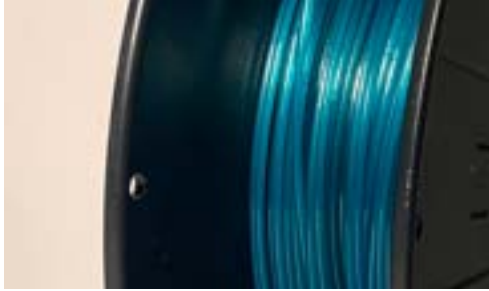
Picture 7: A good example of spooled filament. (25% blue flakes 75% transparent PET flake mix)
