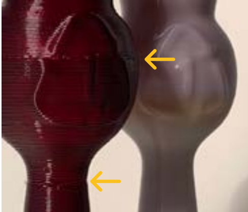
Picture 17: On the left is a print with 2 stoppages. That causes the faulty lines in the model.
