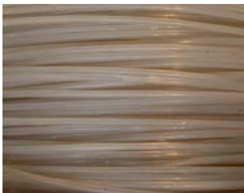
| Picture 7: A good example of spooled filament. Consistent diameter and perfectly aligned.
