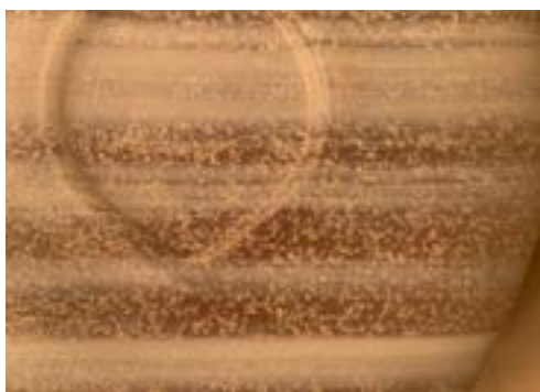
Picture 10: Picture showing an extreme amount of moisture trapped inside the print walls and lines of too little cooling.
