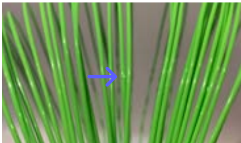
Picture 13: A bad example of spooled filament. You can see a big blob in the middle of the spool.
