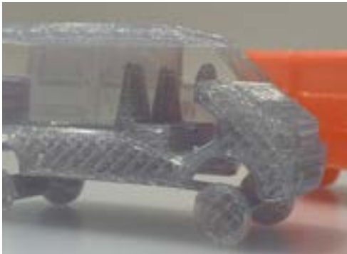
Picture 18: Picture showing an the inside of a print that could not be resumed due to the lack of a filament clog sensor.
