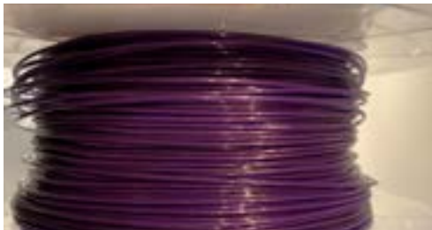
Picture 10: Resulting spool of the mixture of PLA from the image above.
