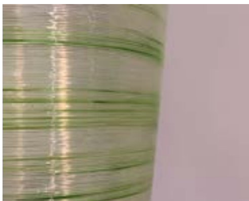
Picture 20: Result achieved by using coloring PLA sparingly in the hopper, giving a striped look to the filament, not found in commercially available PLA.
